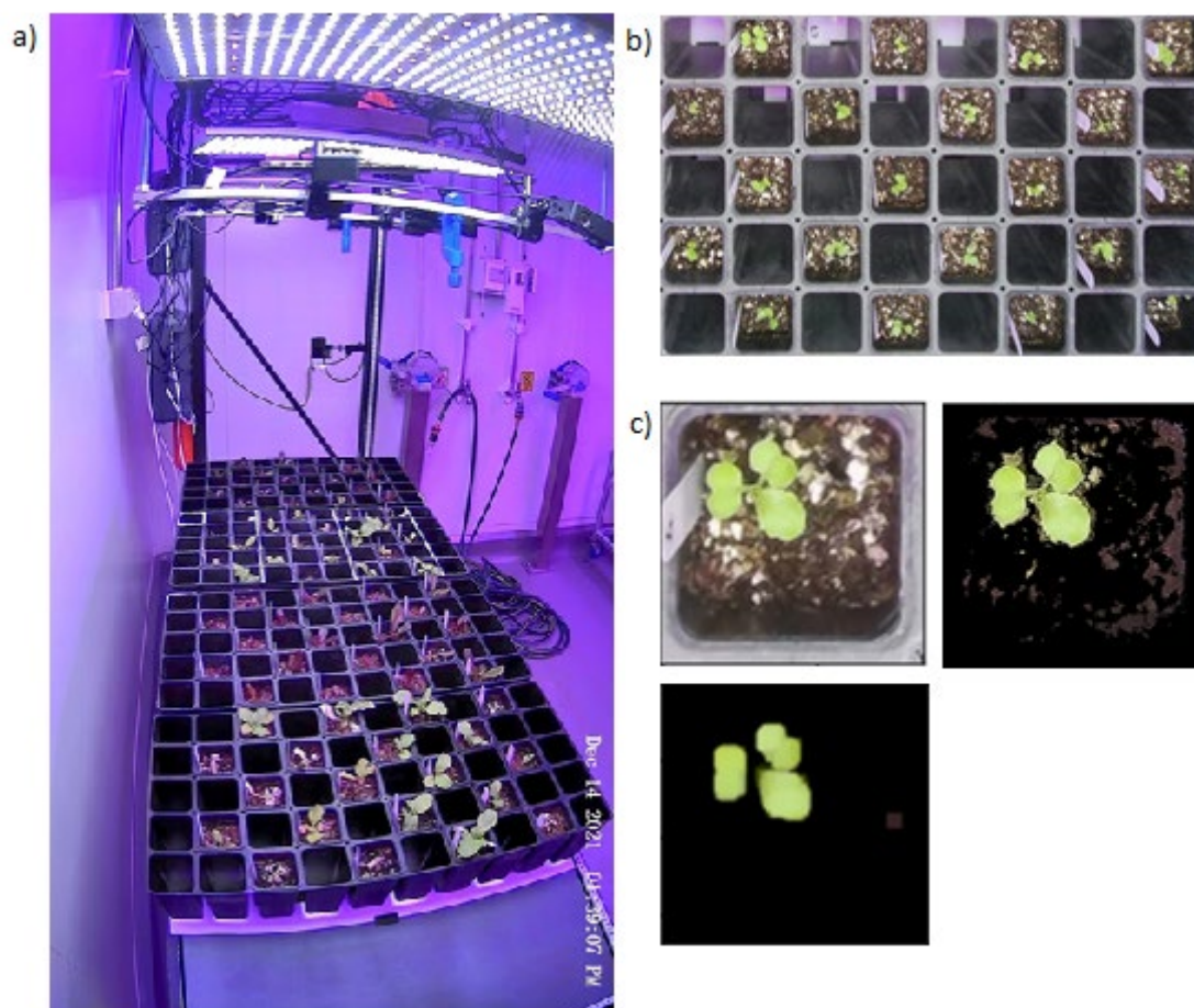
Figure 1. Experimental setup in ground-based laboratory – a) experimental rig, b) top view image from visible colour camera, c) basic image processing to segment plant leaves from the background
